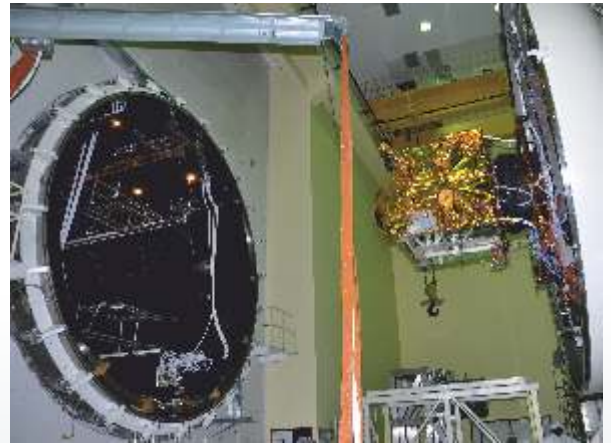
IRNSS-1F being loaded into thermo-vacuum chamber
