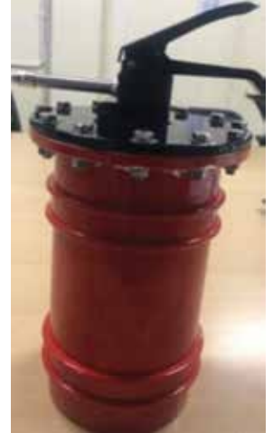
Prototype of Portable fire suppression system
