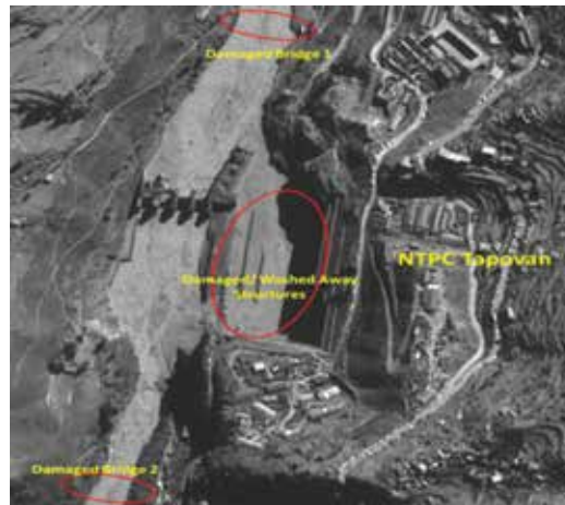
Damage to Tapovan Project due to flash flood in Rishi Ganga River as viewed by Cartosat Satellite
