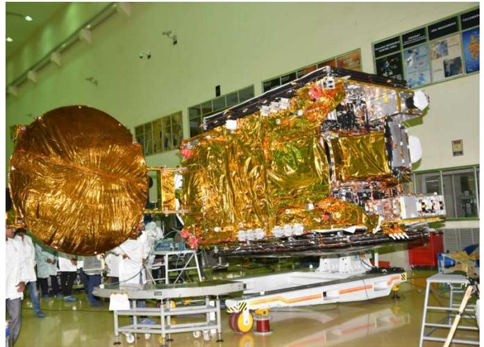
GSAT-31 Antenna Reflector Deployment test
