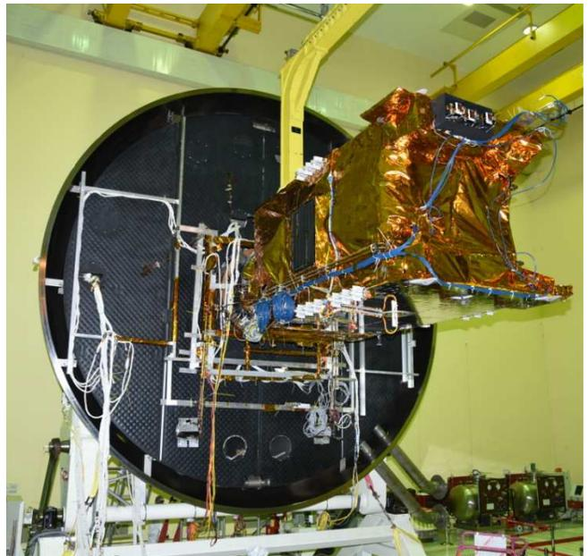
Loading of GSAT-31 into Thermovacuum chamber
