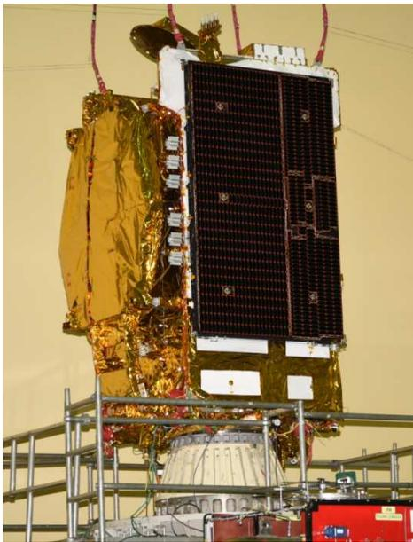
GSAT-31 during Vibration Test
