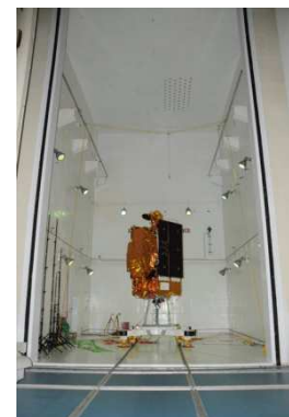
GSAT-7A undergoing Acoustic Test
