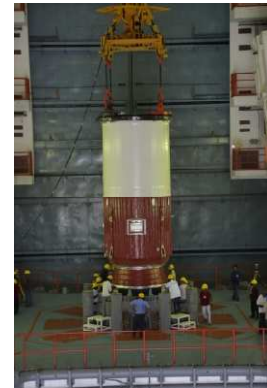
Placement of Nozzle end segment of GSLV-F11 Core stage
