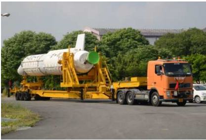
Liquid Strap-on (L40) being transported to Vehicle Assembly Building
