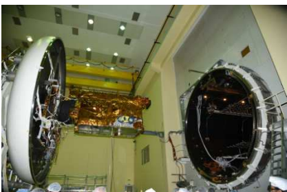
GSAT-7A being loaded into Thermovac chamber
