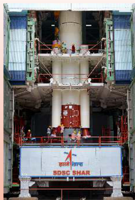
Integration of strap-ons to PSLV-C35 core stage at Mobile Service Tower
