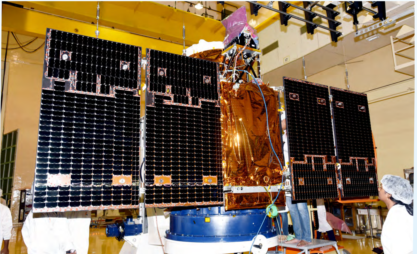
Cartosat-2 Series Satellite undergoing solar panel deployment test
