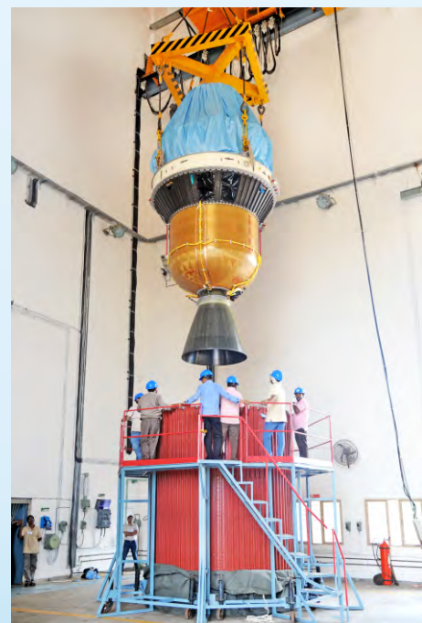
Assembly of third and fourth stages of PSLV-C38 at Stage Preparation Facility
