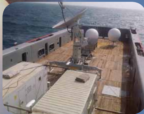
An Indian ship carrying dish antenna to monitor the flight of PSLV-C25
