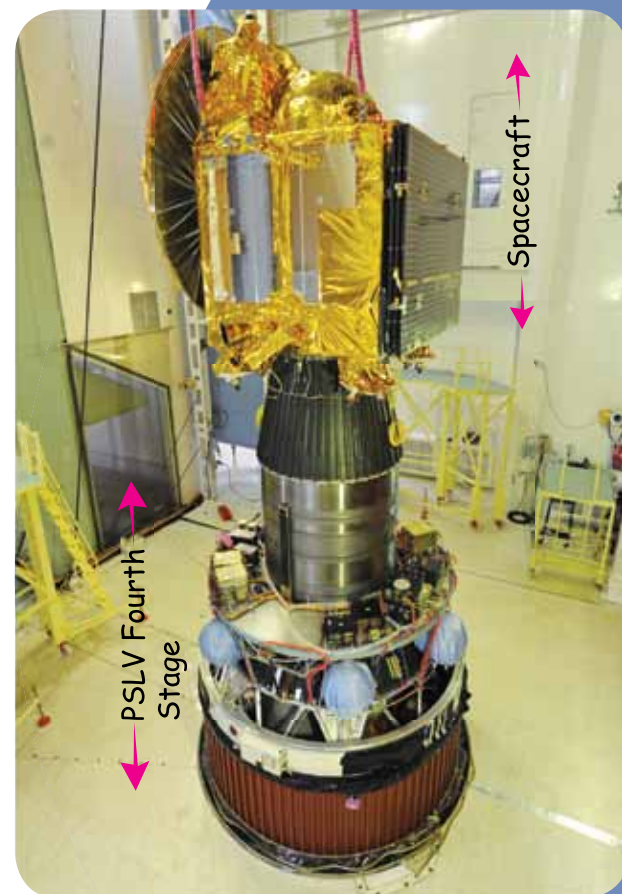
Mars Orbiter Spacecraft mounted on top of PSLV-C25 fourth stage
