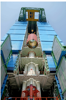
Hoisting of an interstage during PSLV-C44 integration
