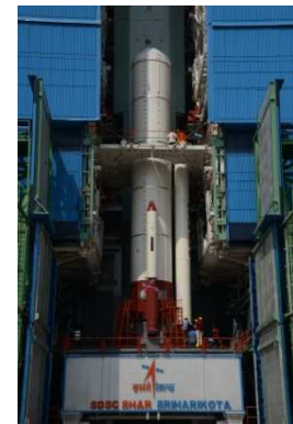
Integration of strap-ons of PSLV-C44 with the core stage
