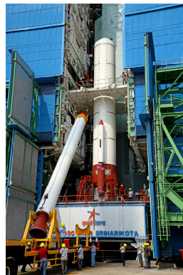
Hoisting of one of the Strap-ons of PSLV-C44 during vehicle integration
