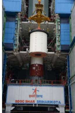
Placement of nozzle end segment of PSLV-C44 core stage
