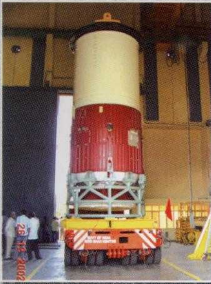
Nozzle-end segment of S139 motor along with Core Base Shroud (S139 motor comprises 5 segments)
