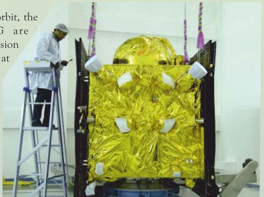
IRNSS-1G in clean room at SDSC SHAR
