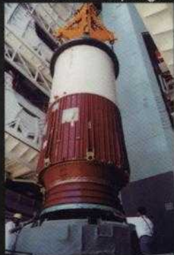
Core Base Shroud + Nozzle End Segment
