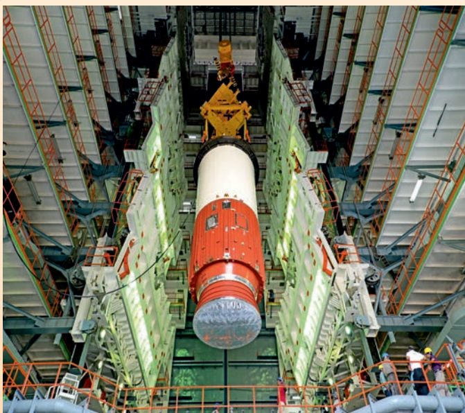
Nozzle End Segment of PSLV-C39 core stage being hoisted over the Mobile Launch Pedestal during vehicle integration
