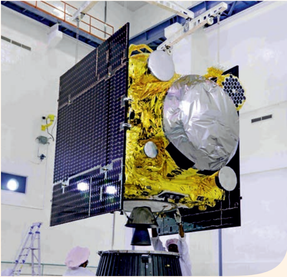
Hoisting of IRNSS-1H during its integration with conical adapter
