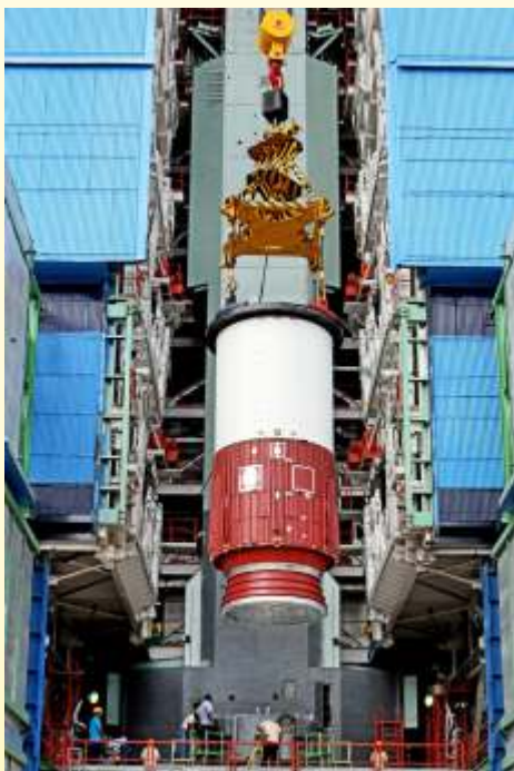
Hoisting of PSLV-C40 core stage nozzle end segment during vehicle integration
