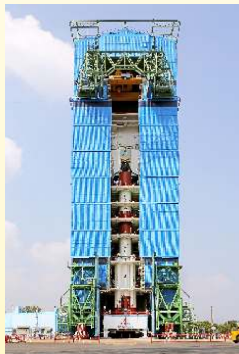
PSLV-C40 integrated upto fourth stage inside Mobile Service tower
