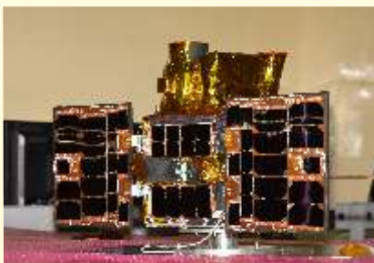
INS-1C with its panels in deployed condition
