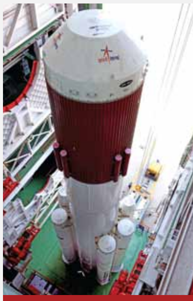
PSLV-C22 first stage with strap-ons inside mobile service tower
