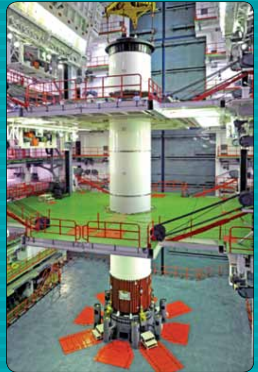
GSLV-D5 core stage integration at Vehicle Assembly Building
