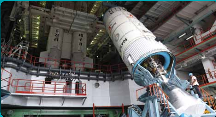
GSLV-D5 second stage being transferred to the Vehicle Assembly Building
