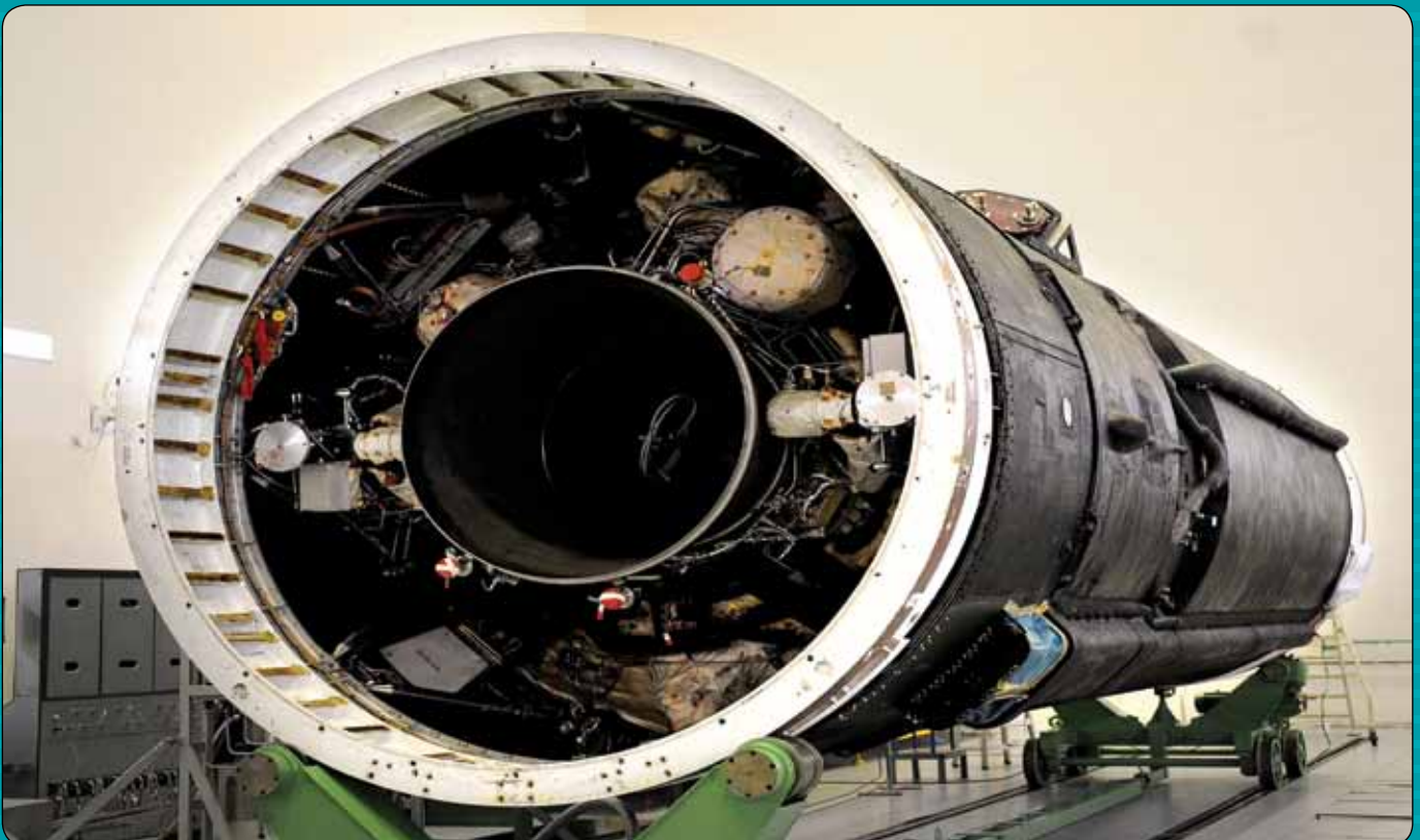
Indigenous Cryogenic Upper Stage of GSLV-D5
