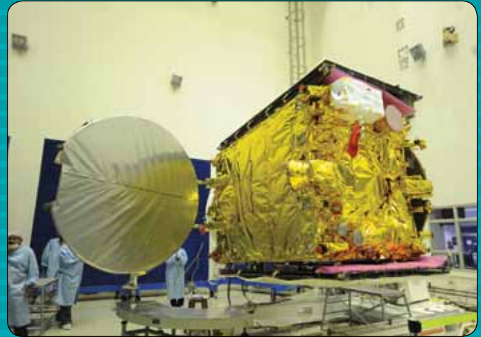
Close-up view of GSAT-14 in clean room
