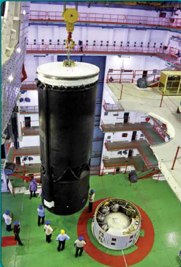
Cryogenic stage integration to the vehicle in progress
