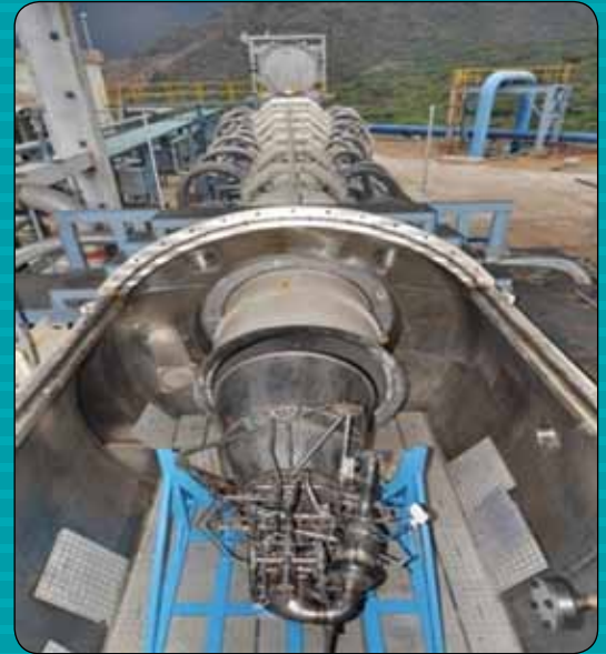
Cryogenic Engine being tested at High Altitude Test (HAT) facility
