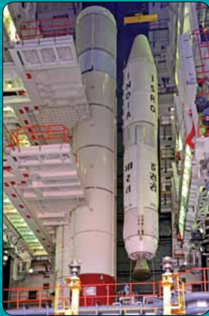
One of L40 Strap-ons being assembled to the core stage
