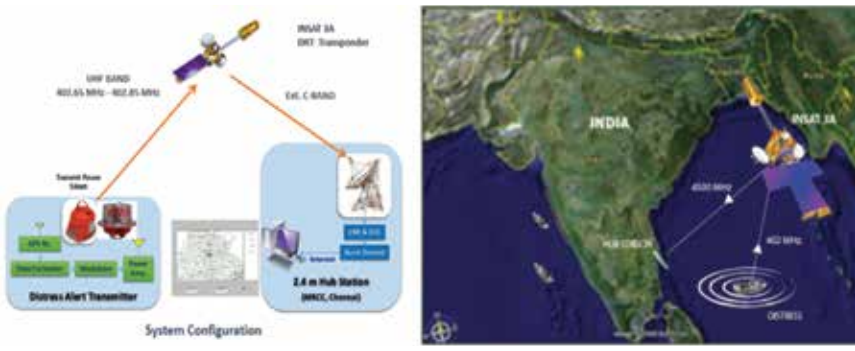
Figure 4. A typical system of distress alert system.
