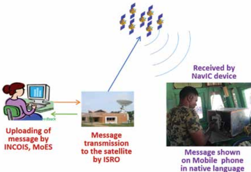
Figure 4: NavIC Messaging System Architecture
