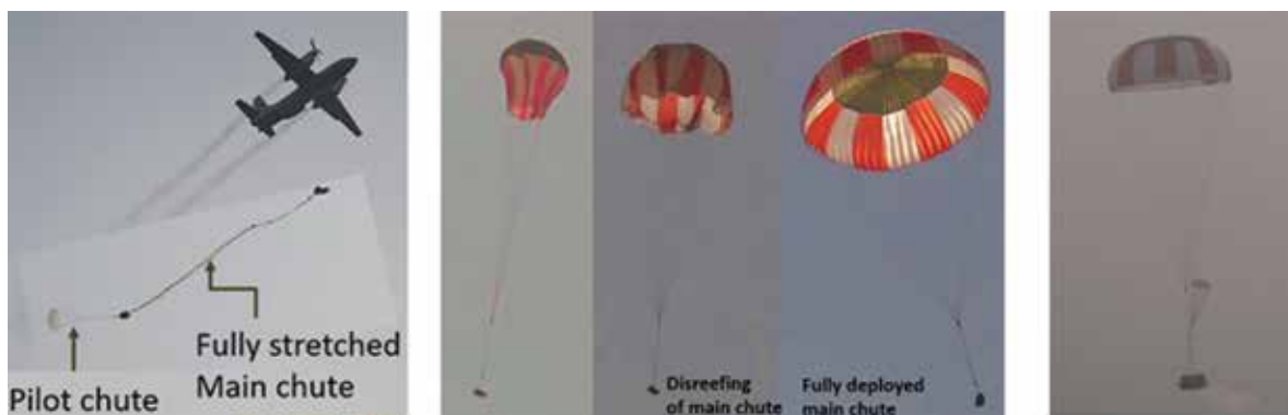
AN32 IL-76 Aircraft drop tests and Main Parachute inflation
