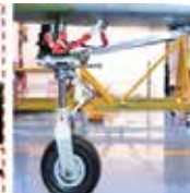
Landing Gear: Qualification of Nose Wheel Steering Actuator and MLG Brake Actuator
