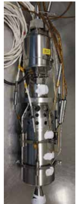
Green mono propellant based 100 N RCS thruster
