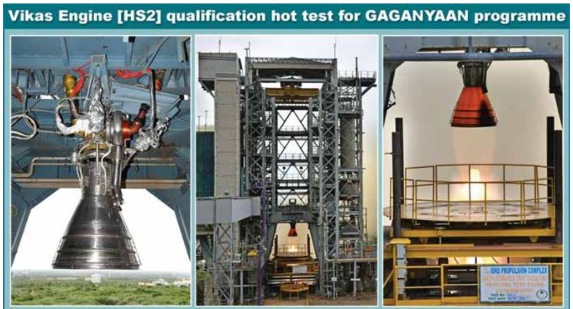
HS2 GAGANYAAN long duration hot test at PTS
