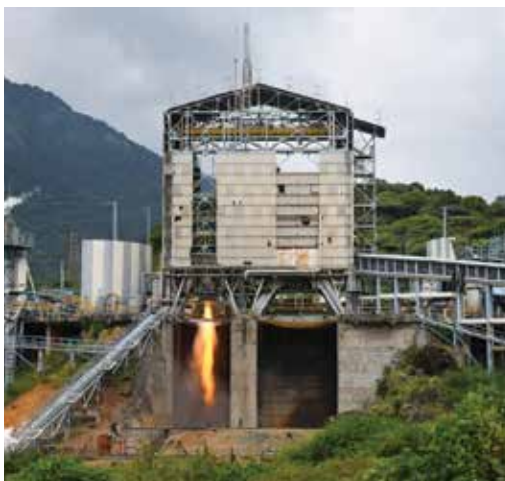
CE 20 Engine Hot Test
