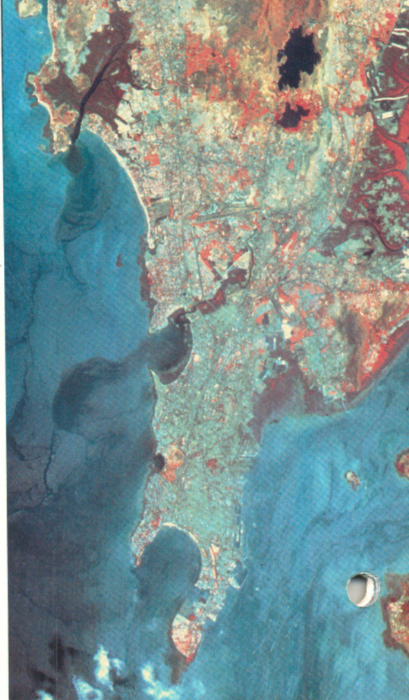
False Colour Composite of a special product of Bombay generated after histogram modification using gaussian
