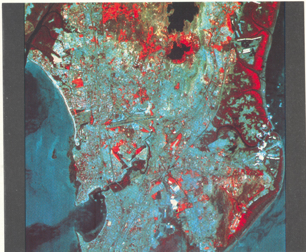
A portion of the Bombay imagery generated after reducing the noise and stretching the data for enhancement of contrast.
