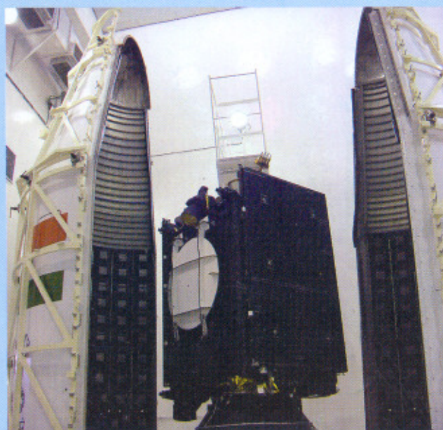
GSAT-2 spacecraft before payload fairing closure
