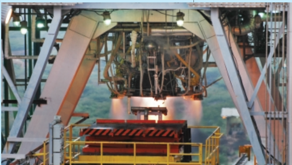
Flight Acceptance Hot test in progress
