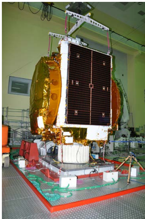
GSAT-17 Undergoing Vibration Test
