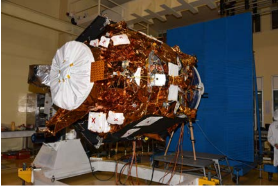
Cartosat-2 Series Satellite undergoing EMI Radiation Test
