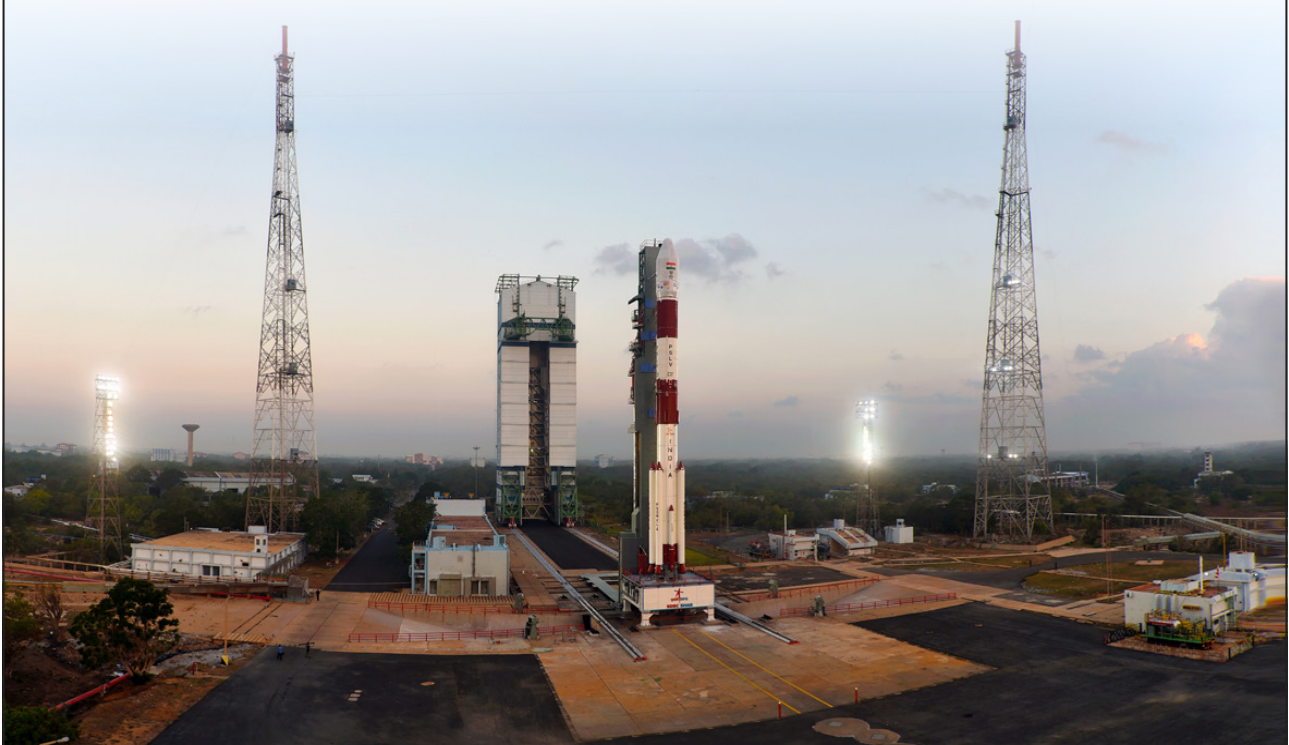
Fully Integrated PSLV-C37 seen with Mobile Service Tower
