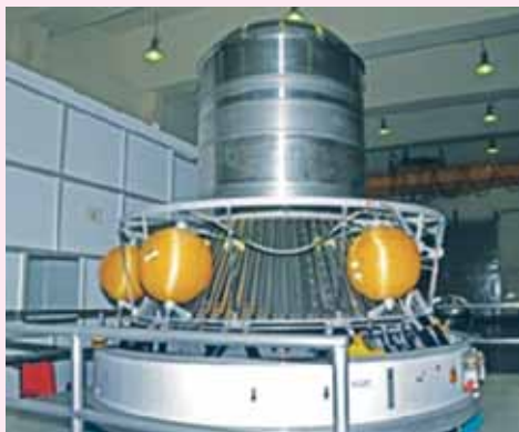
Liquid Upper Stage of PSLV
