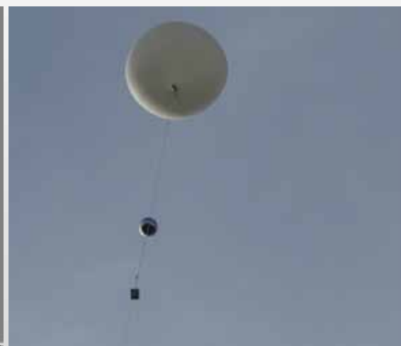
The DWR, Cherrapunjee coverage for elevation angle of 3 degree (left). Calibration of the DWR using metal sphere attached to hydrogen gas filled balloon & Pisharoty sonde (right)
