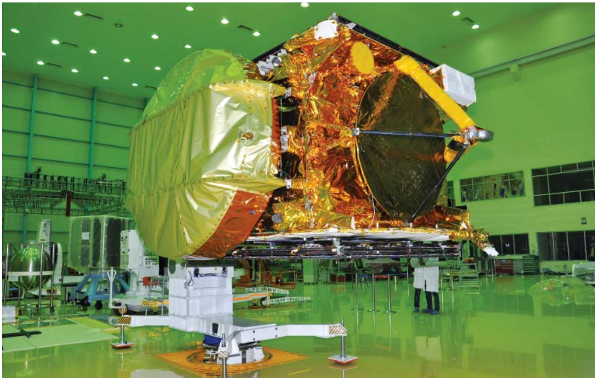
GSAT-16 in clean room undergoing pre-launch tests
