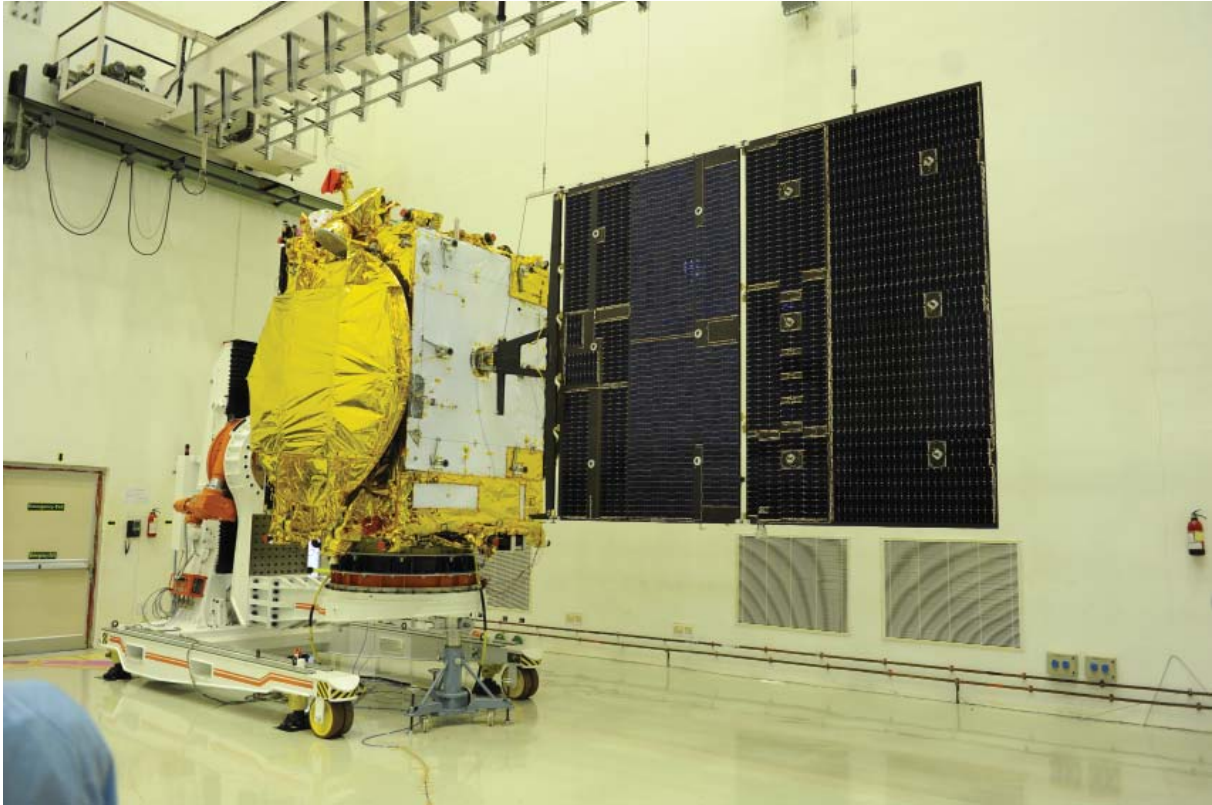
GSAT-14 in clean room with one of its solar panels deployed
