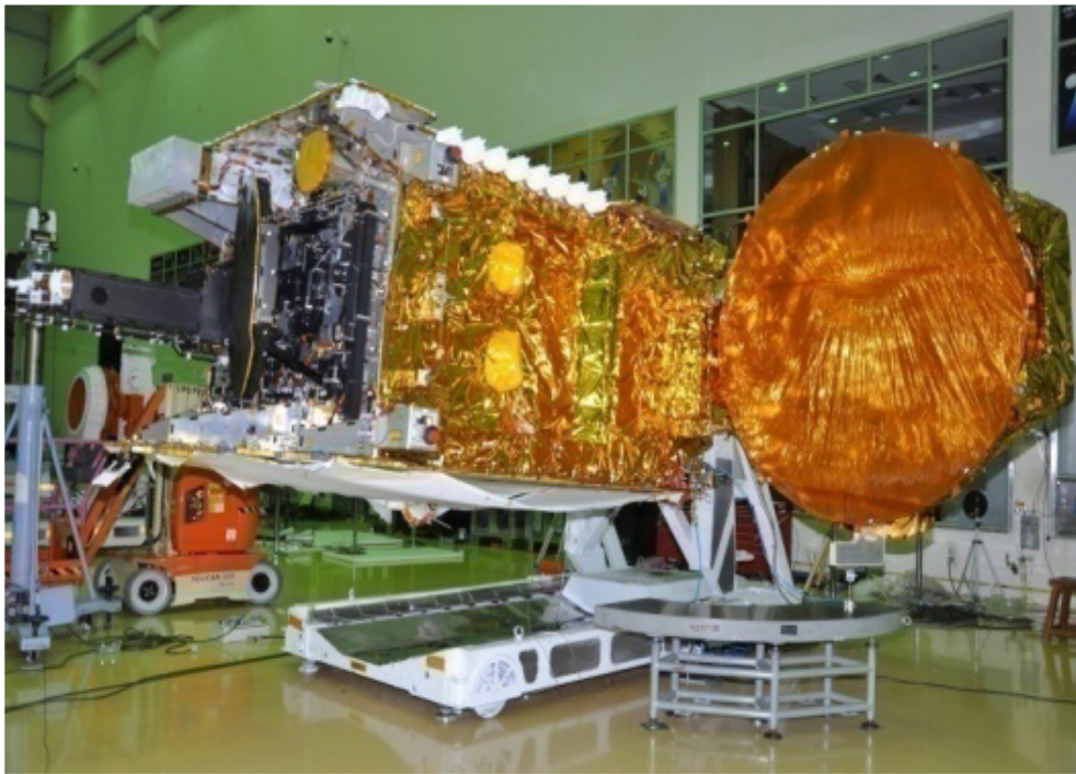
GSAT-18 undergoing Reflector Deployment Test
