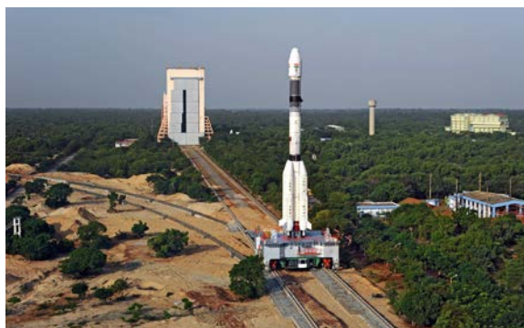
Panoramic View of GSLV-F05 being moved from Vehicle Assembly Building (VAB) towards Launch Pad
