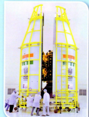
INSAT-3DR Integrated with GSLV-F05
