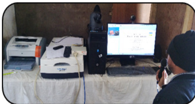
Telemedicine node with videoconferencing and medical diagnostic instruments
