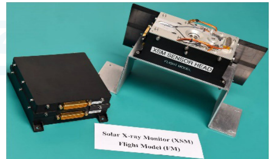
Photographic view of XSM payload Flight Model (Left - XSM Processing Electronics package, Right - XSM sensor package).
