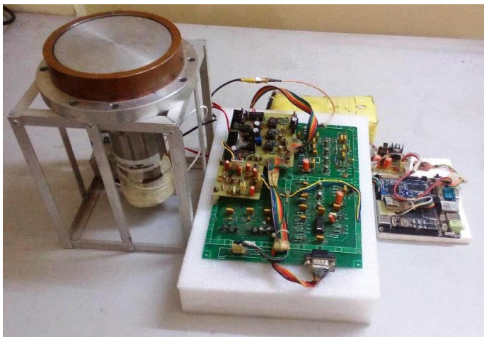
5" dia phoswich detector being tested Fig 7b
