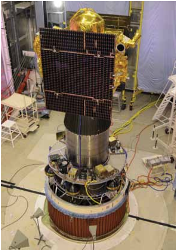
IRNSS-1D integrated with the fourth stage of PSLV-C27
