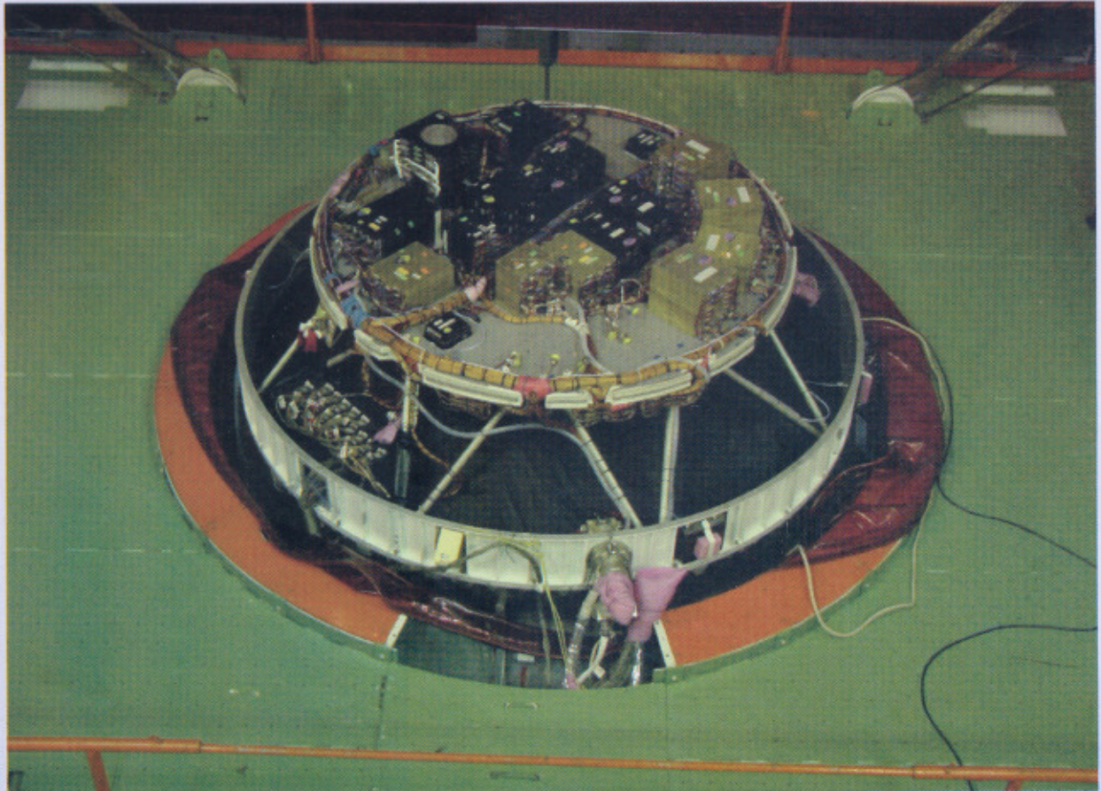
Equipment Bay – The 'brain of GSLV-F01
