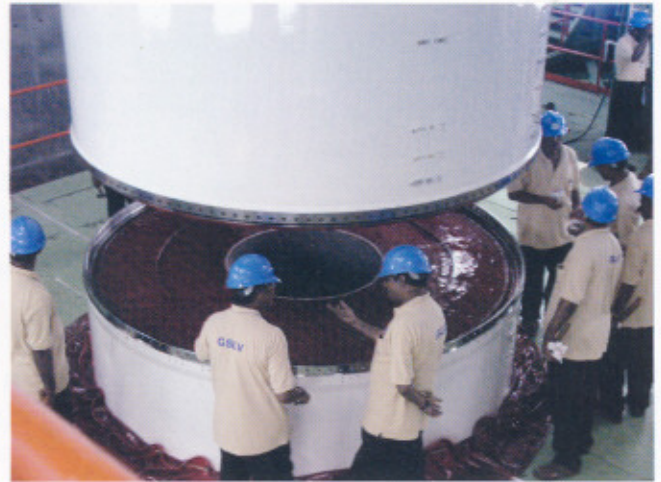
Integration of GSLV-F01 first stage segments
