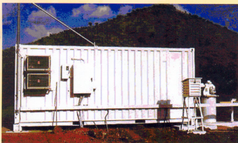
GONG telescope and shelter. The Telescope is seen at the extreme right of the picture mounted on a white cylindrical pillar. The shelter houses a sophisticated Michelson Interferometer which is the heart of the instrument used for precise velocity and magnetic field measurements
