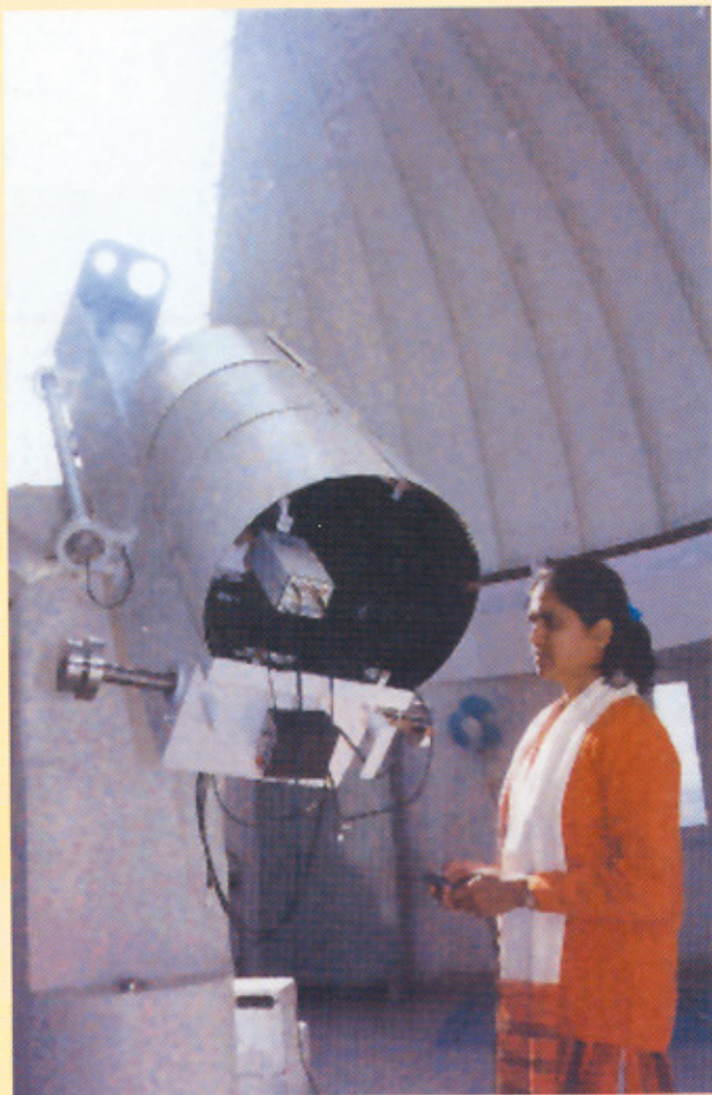
Spar Telescope carrying the 15 cm achromatic lens as the objective (seen at the far-side), while the CCD camera that records the images is seen at the back-end of the telescope
