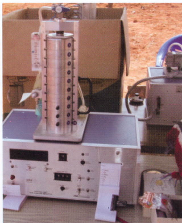
Quartz Crystal Microbalance used for aerosol and mass concentration study
