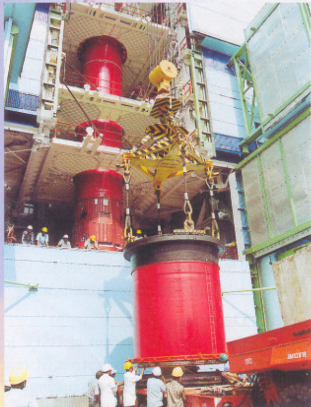
Integration of GSLV Core stage segments.
