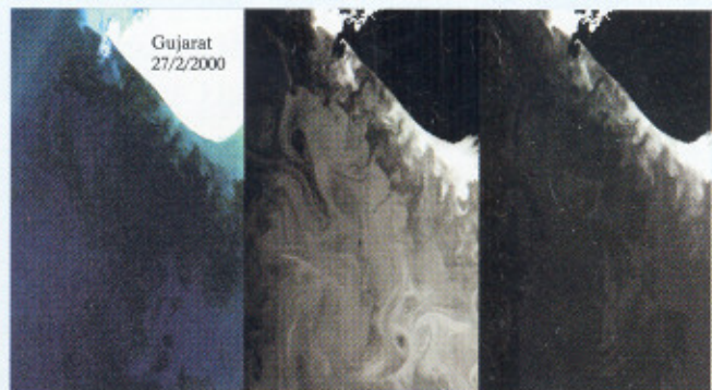
Effects of atmospheric correction of IRS-P4 OCM data in band 3 and band 5
