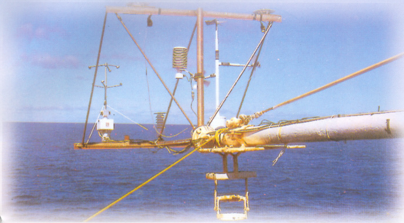
The Experimental arrangement on board Sagar Kanya for boundary layer measurements.
