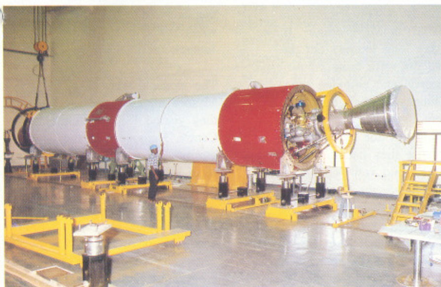
L-40, the Liquid Propulsion Strap-on stage of GSLV which was successfully tested on March 5, 1998.
