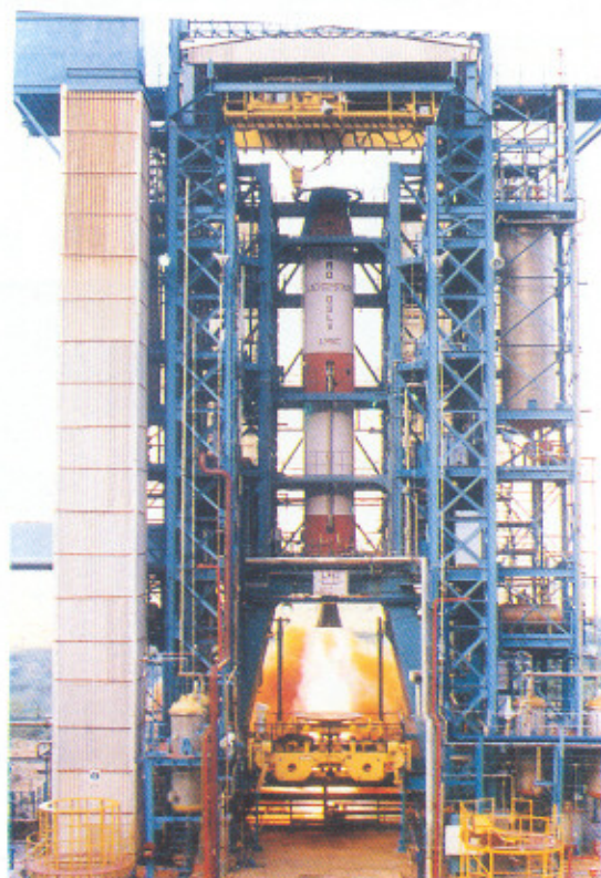
L-40, GSLV Strap-on Liquid Propellant Motor under test
