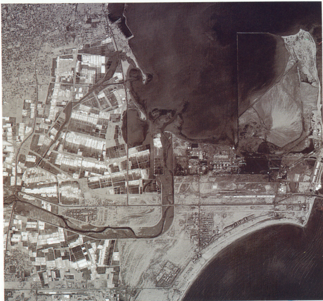
Picture taken by the Panchromatic Camera (PAN) of IRS-1D on October 7, 1997 showing part of Tuticorin Town in Tamil Nadu. The picture which has a 5.8 metre ground resolution clearly shows rectangular salt pans. The regulated drainage system can also be seen besides built up structures.
