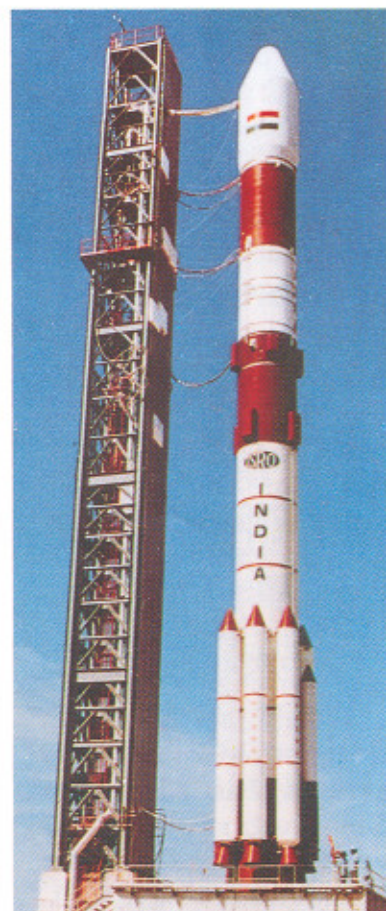
India's PSLV launcher uses six solid strap-ons. The next-generation GSLV introduces a cryogenic third stage and adapts the PSLV's second-stage liquid engine technology for its strap-ons.
