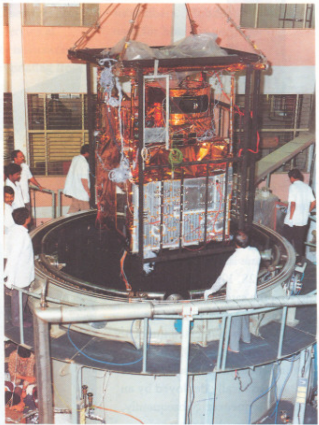
IRS-1C being loaded for thermovac test
