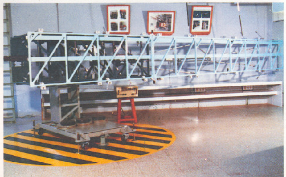
Full size SAR antenna with one wing deployed
