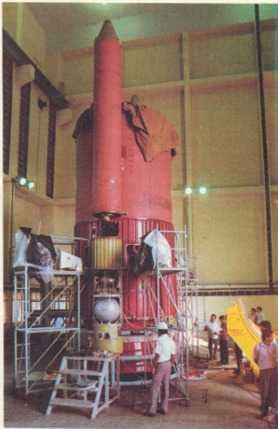
SITVC and Reaction control thruster along with PS-1 nozzle end segment at the Solid Motor Preparation Facility
