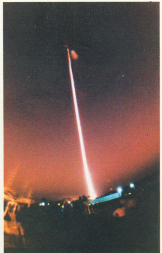
RH-560 lift-off and the release of multiple Barium blobs, as a part of the 'Ionisation hole' experiment
