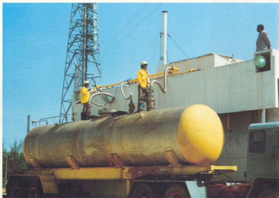
N 2 O 4 tanker being interfaced with the fluid circuits
