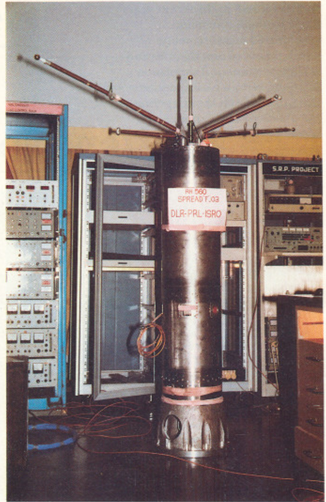
ISRO-DLR Experiment for study of day-time equatorial F-region with deployable booms
