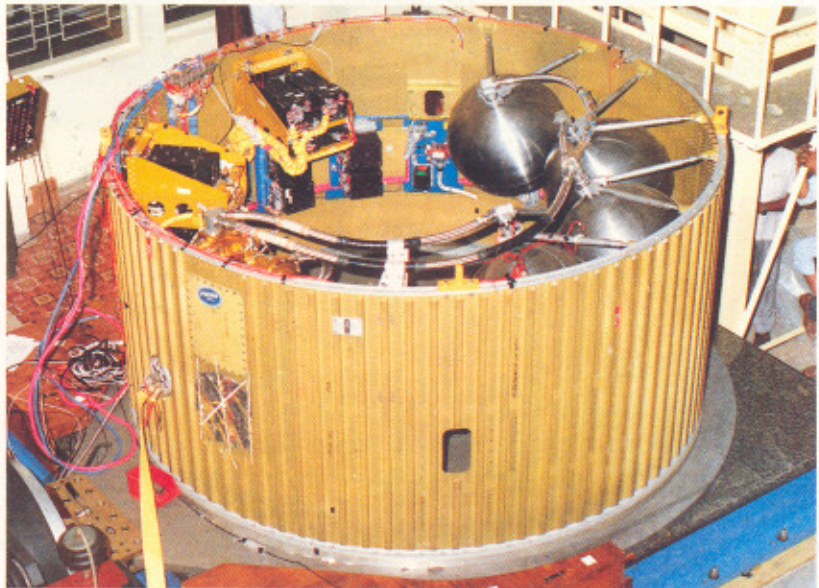
Inter-stage between second and third stages (2/3 L)
