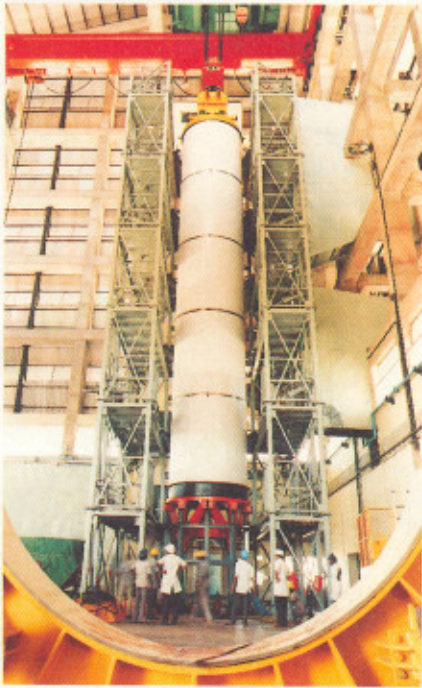
The five-segment first stage solid booster
