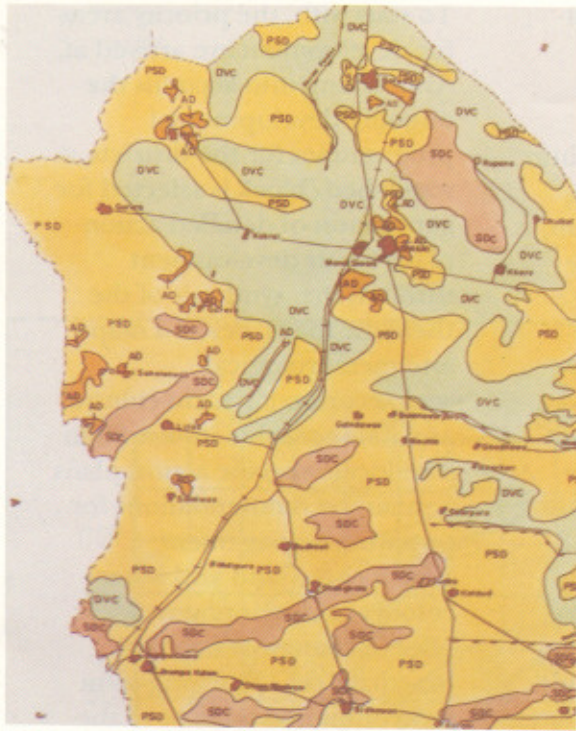
Geomorphological map showing landforms — Active Dunes (AD), Partially Stabilised Dunes (PSD), Stabilised Dune Complex (SDC) and Dune-Vale Complex (DVC)
