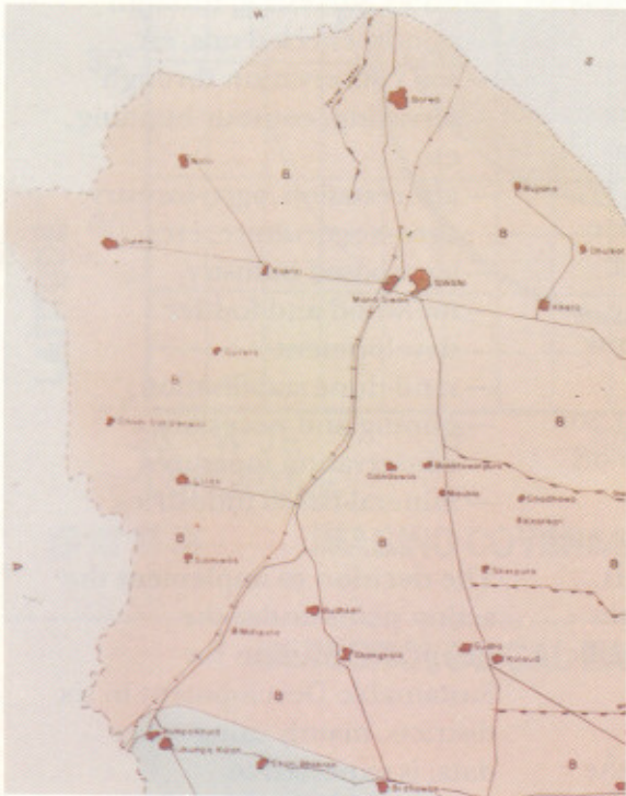
Ground water quality map showing highly saline (8), fresh in shallow and sodic in deep depths (5)
