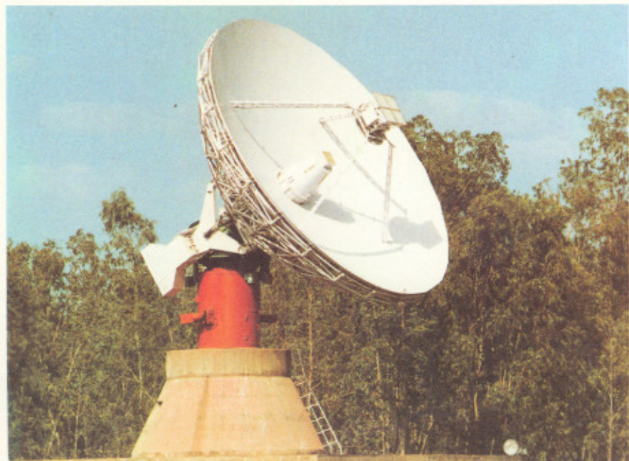
S-band Telemetry Antenna
