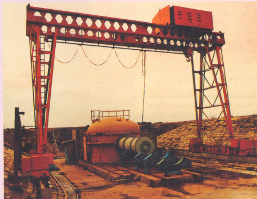
PS-3 static test bed at SHAR Centre
