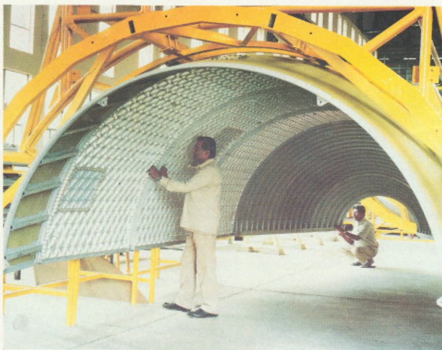
PSLV heatshield under inspection
