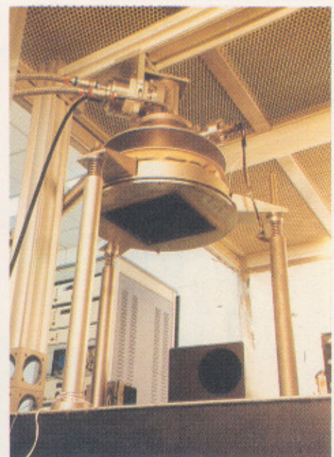
Bench cooler cryo surface
