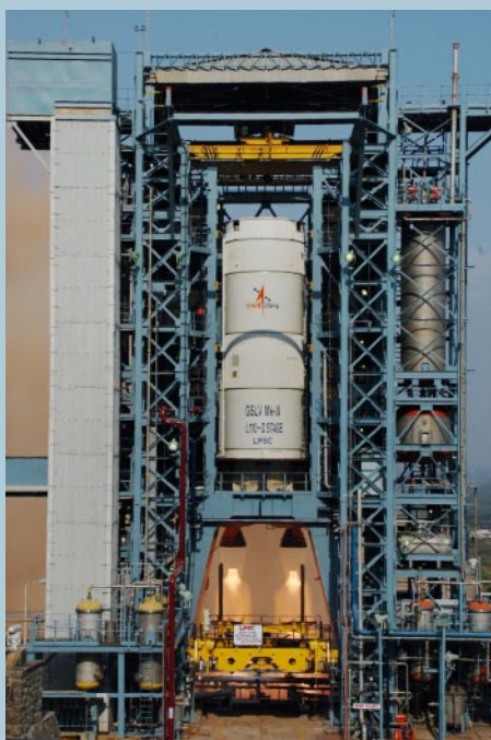
Static Testing of L110 Liquid Core Stage
