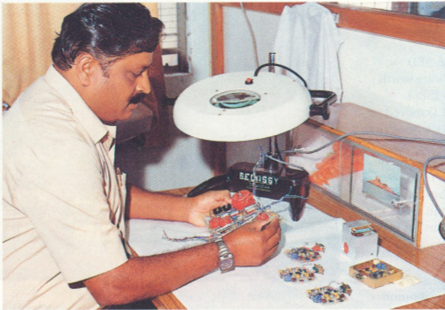
Inspection of wired assemblies after conformal coating.
