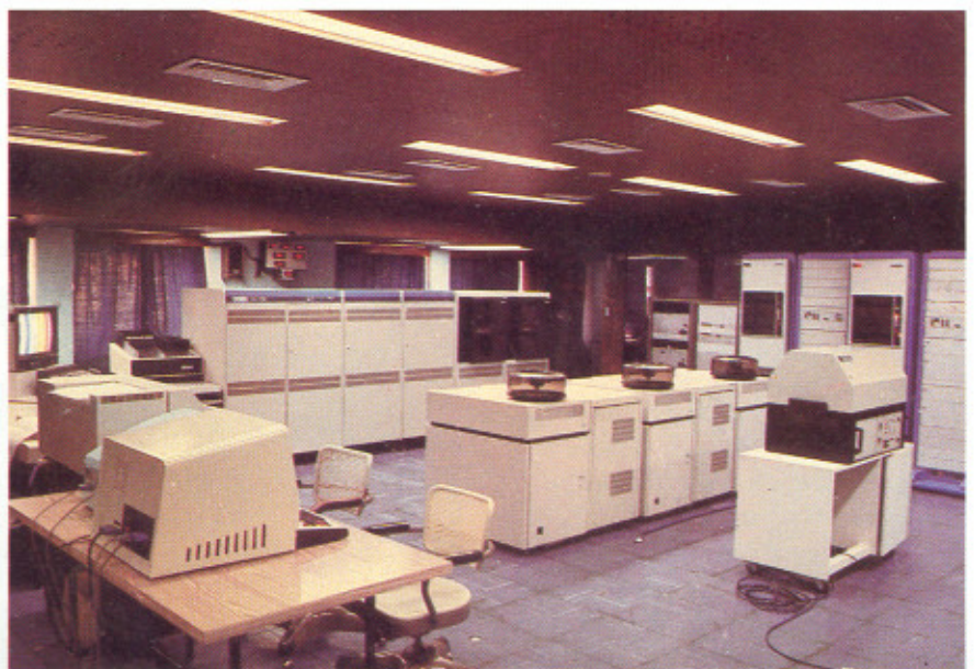
Vax-11/780 Computer used in NRSA for image processing.
