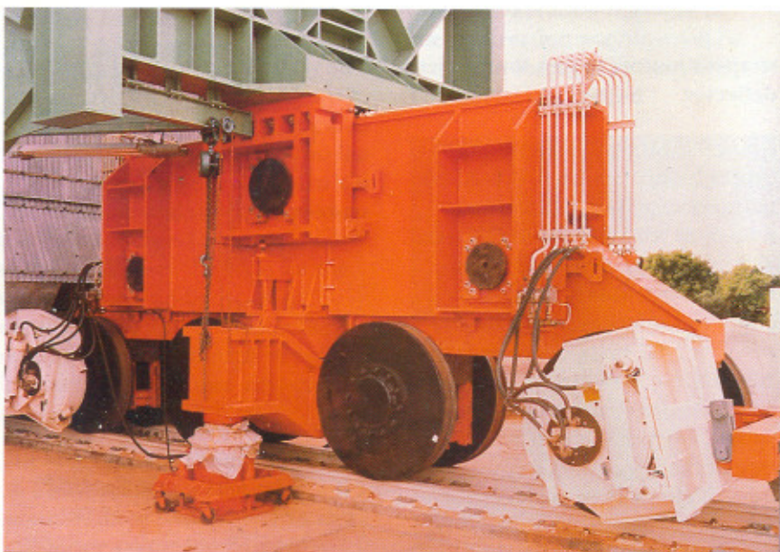
The wheel bogie system of MST - A powerful puller.
