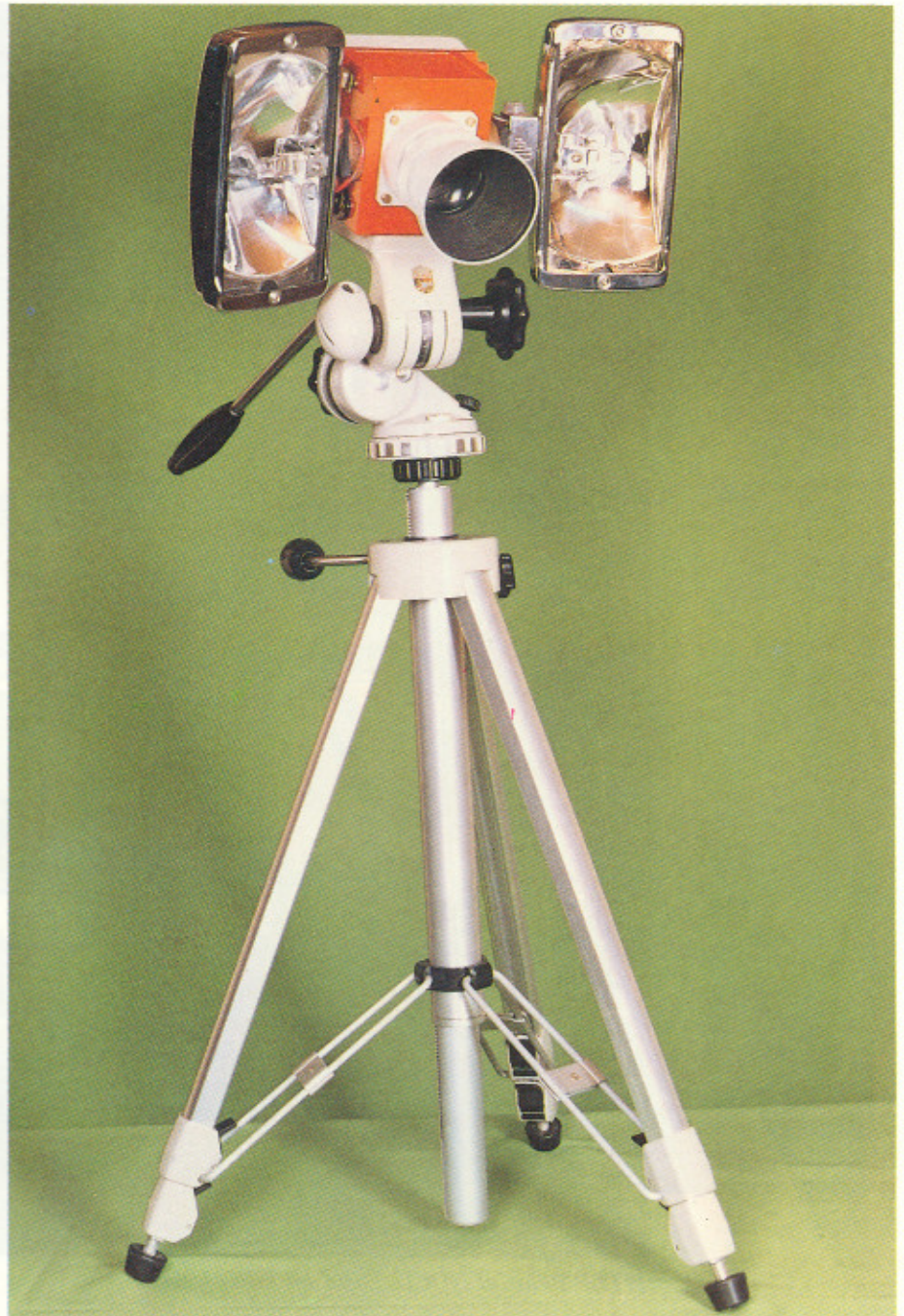
Hygrophotometer for measurement of moisture content in plant leaves – Technology transferred from ISRO
