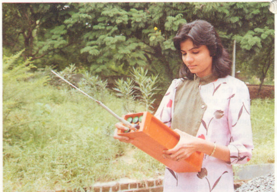
Personal locator beacon - technology transferred from ISRO.
