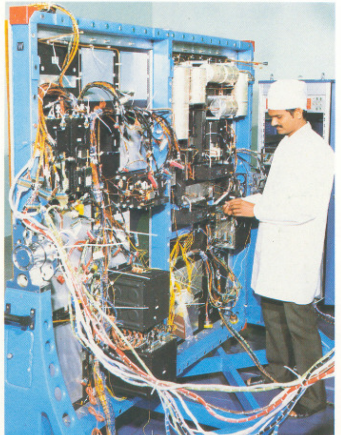
Communication payload for INSAT-II TS.
